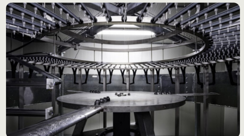
Top: Airflow analysis in our wind tunnel Bottom: Our in-house rain erosion test rig
