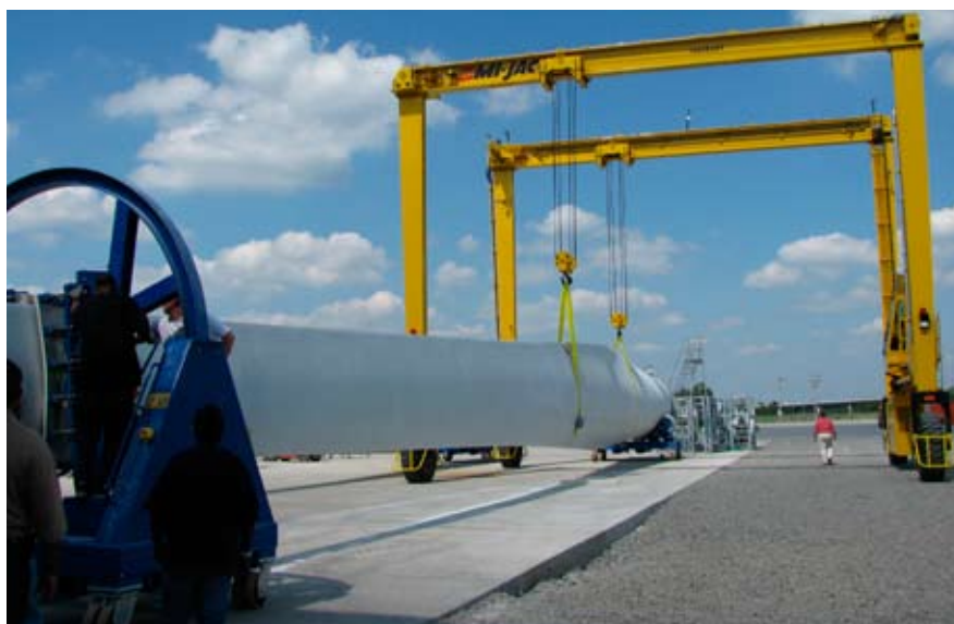
The yellow gantry crane in Little Rock is able to handle even our largest blades. The picture shows the first LM 43.8 produced in Little Rock being moved to the storage area.
