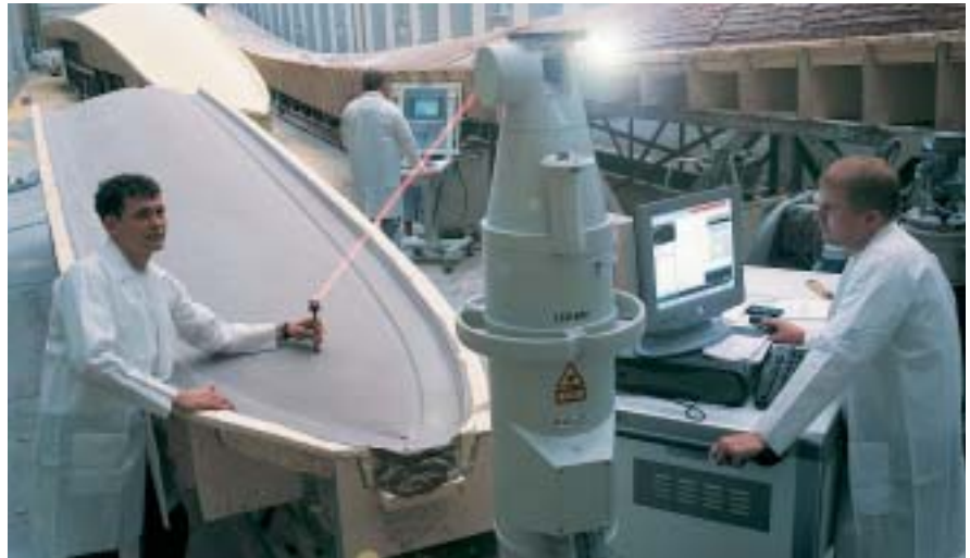
Laser measurements used to check the plug. An accurate measuring technique is a prerequisite for complying with quality standards.
