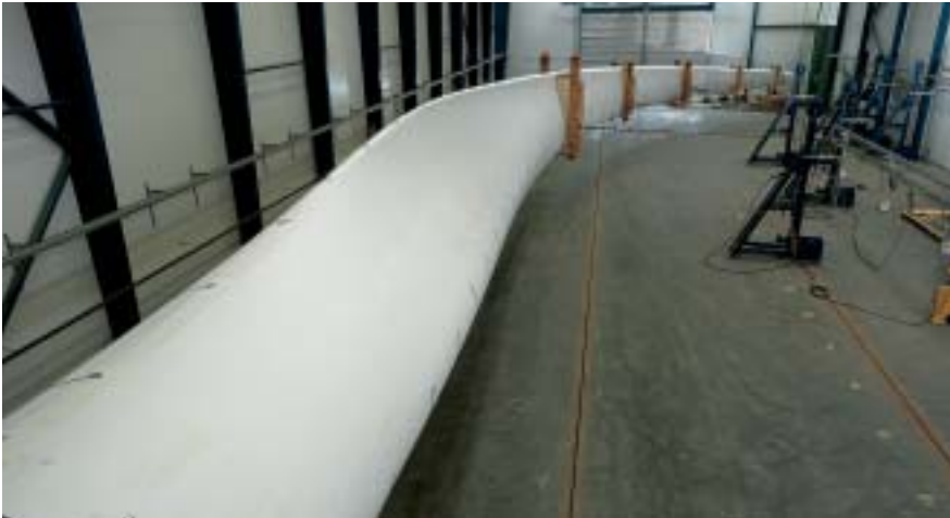
The blade undergoes a static test as part of the test programme – the deflection at the tip of the blade was approximately 16 metres during this test.
