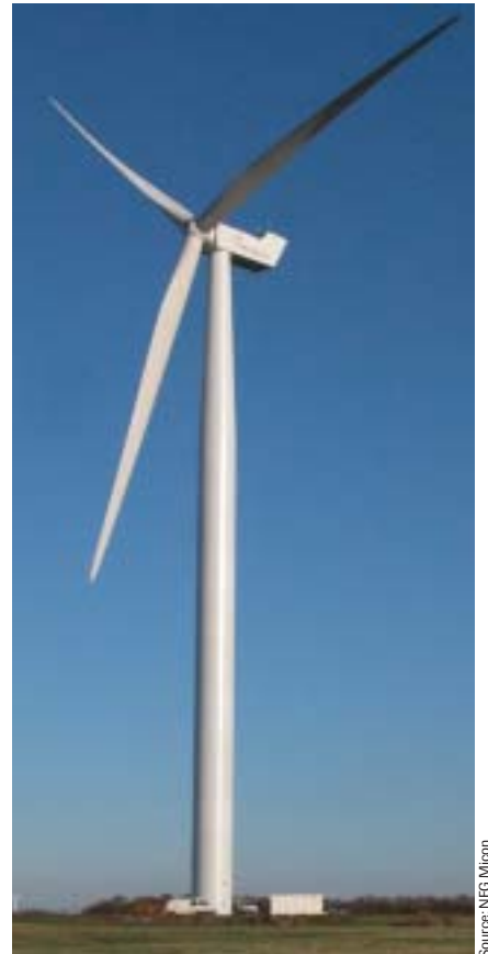
The LM 54.0 P blade is now turning on a 4.2 MW NEG Micon test turbine
